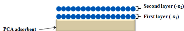
Fig. 3. Schematic representations of the formation of two layers on the PCA surface.
